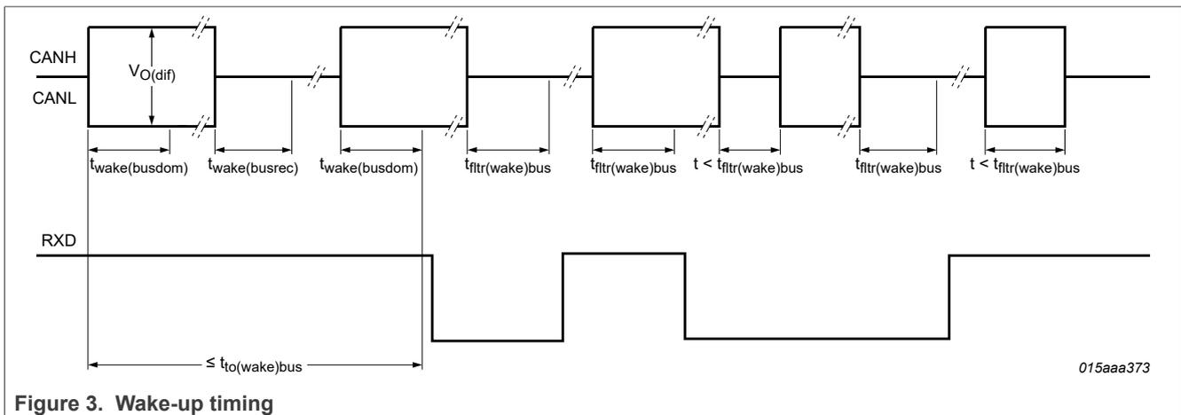
Figure 3. Wake-up timing
